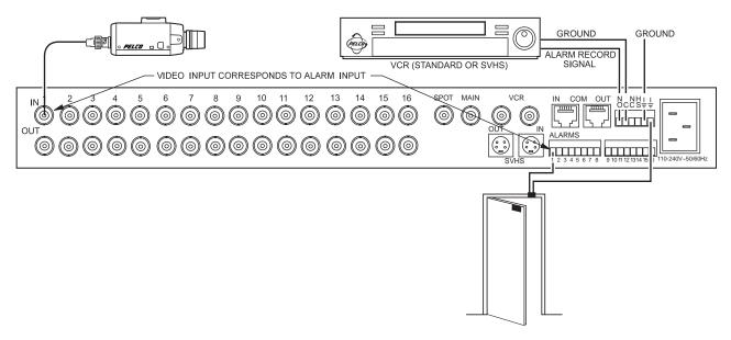
Figure 8. Alarm Wiring Example
